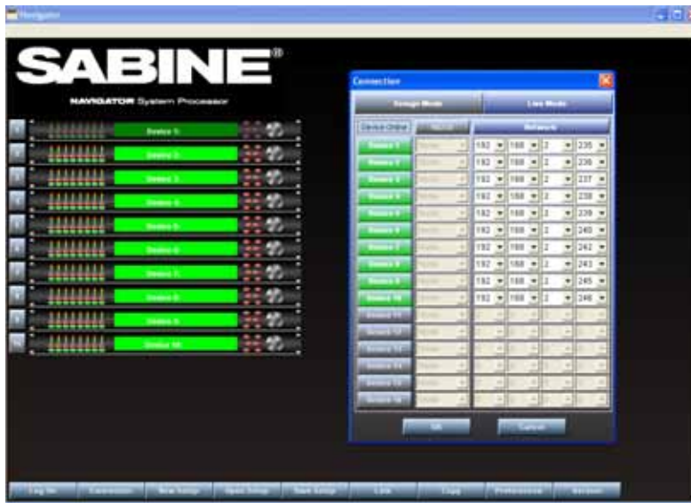
Main screen in Navigator Software, showing Connection window with IP addresses assigned and 10 devices present. Device 1 is not connected.
